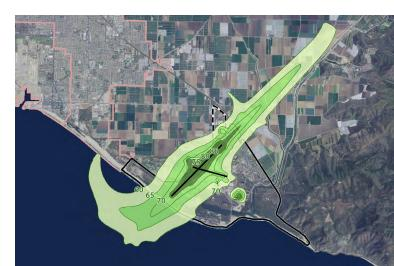
Noise contours are lines or "footprints" of noise levels drawn around a noise source.
