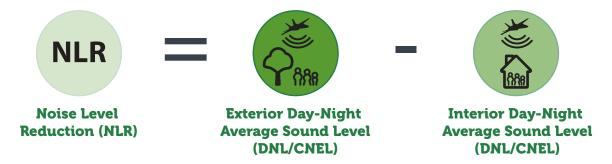
Sound travels from the exterior to the interior of a building by penetrating the building perimeter through the building's solid structural elements or via openings. Openings in the building (which provide air infiltration paths through windows, vents, and gaps) allow sound to travel directly into the building's interior. Basically, any place that air enters a home, sound will also enter.
