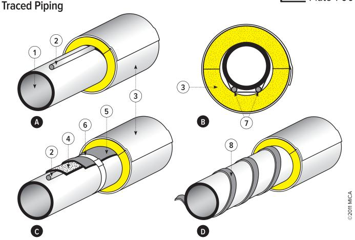
Tracers provide heat for piping which must be protected from freezing, and for process piping which must be maintained at a minimum temperature. The two most common types are (1) tubing which runs horizontally along the length of the piping, and (2) electrical cables or tape coiled around the pipe. Tracers may be thermally connected to the pipe by means of heat transfer cement, or simply banded to the pipe.
