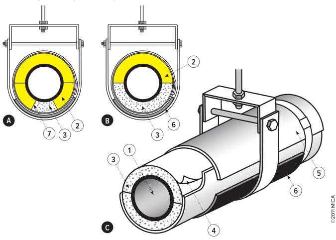
Hot and cold piping insulated with a low density pipe insulation often requires an insert of high density insulation at points of support to prevent the weight of the pipe from crushing the insulation. These inserts may be any one of the high density insulations used for high temperature installations such as calcium silicate and perlite, or any one of the various cellular and foam insulations used on cold applications.
