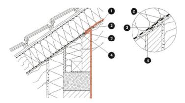
**Fig. F.14** Eaves – above rafter insulation, continuous rafters, lined compartments: (1) air barrier, (2) tape, (3) adhesive, (4) smoothed lining at the crown of the wall
