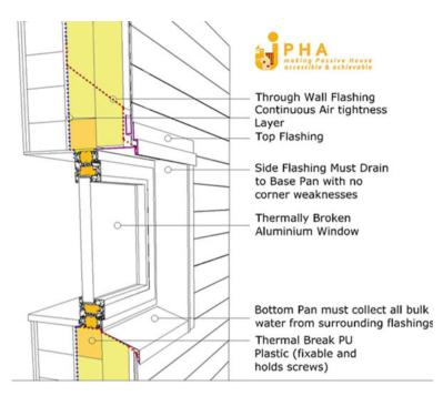
Fig. E.9 Passive House detail of window installation (provided by the Passive House Academy)
