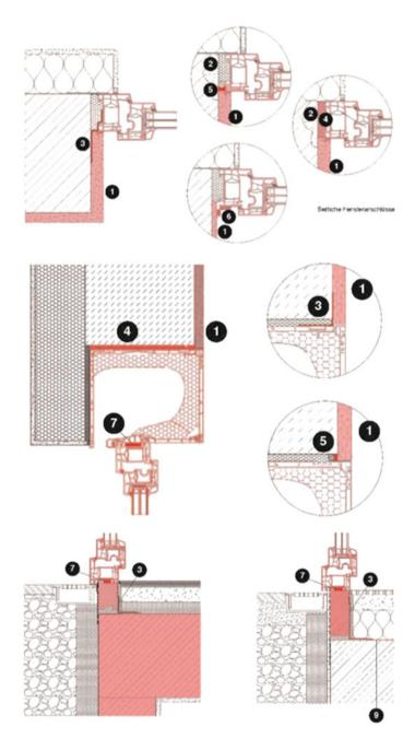
**Fig. F.24** Floor-length windows, French doors in the wall: (1) interior plaster, (2) smooth finish. (If needed) alternatives: (3) foil joint seals, (4) proofed sealant strips, multifunctional sealant strips, (5) spray sealant, (6) bands with sealant strips, (7) sealant for windowsill junction profile for windows, (8) floor recess section, (9) building component sealant
