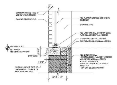
Fig. E.4 Example of thermal bridge in wall construction
