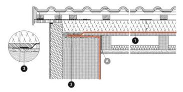
Fig. F.12 Verge – above rafter insulation: (1) air barrier, (2) adhesive
