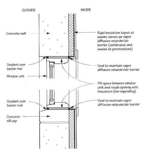
**Fig. E.2** Example of windows installed as part of a barrier wall system. (Illustration taken from Residential Windows: a Guide to New Technologies and Energy Performance)
