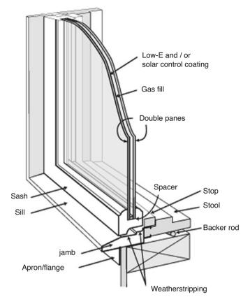
**Fig. 7.1** Typical window and fenestration components. (Not shown are anchoring, wall integration, and other common characteristics.) For a more complete listing of components and definitions, see ANSI/AAMA/WDMA I.S.2
