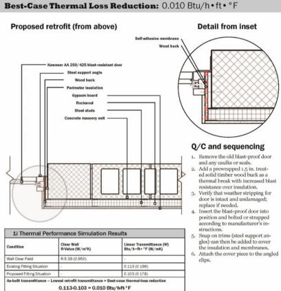
CMU or Concrete Wall with Interior Insulation
