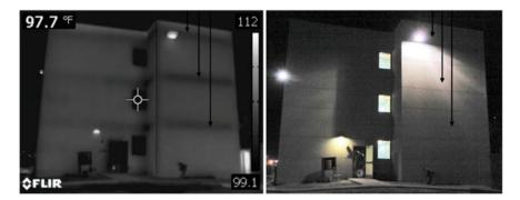
Fig. H4.1 Infrared Thermography image shows loss of thermal barrier continuity due to thermal bridging through exterior wall at floor to wall connections. Note straight anomalies. Source: TMI Air Barrier Testing
