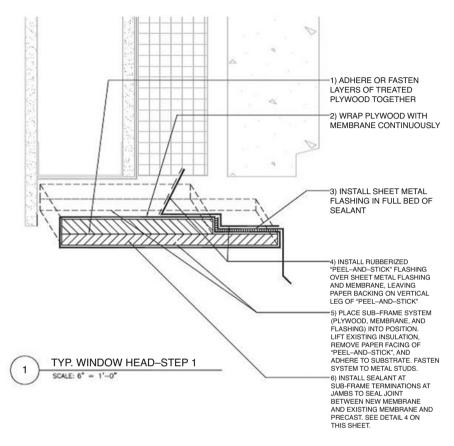
Fig. E.5 Step-by-step illustration of window head installation (Step 1)
