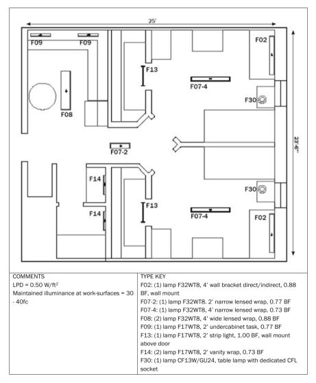
Fig. G.2 Sample schematic lighting layout (not to scale)
