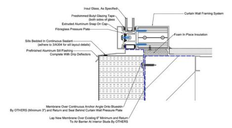
Fig. E.12 Illustration of window installed into EIFS wall
