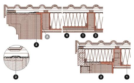
**Fig. F.10** Verge – between-rafter insulation sub-top: (1) air barrier, (2) adhesive, (3) supporting lath, (4) protection layer (optional)
