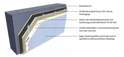
(1) Existing wall; (2) first mineral wool insulation layer (boards) to prevent thermal bridges; (3) metal or wooden studs as substructure, flexible mineral wool batts in between; (4) vapor barrier with flexible density (smart vapor retarder); (5) gypsum boards, open to diffuse
