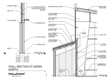
Fig. F.33 Pre-engineered metal wall systems
