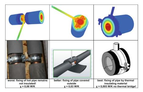
**Fig. 8.9** Fixings of hot pipes are worthwhile to be well insulated (example: 20-mm pipe with insulation 1\*DN): large heat losses because of high temperatures of pipes. Source (AKKP 49)
