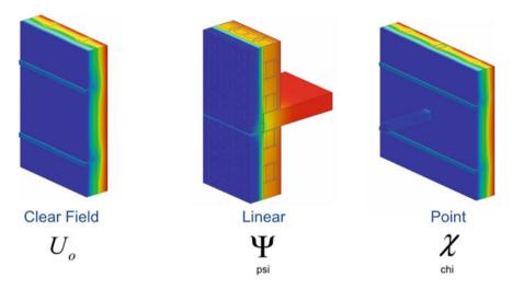
Fig. 8.11 Types of transmittances
