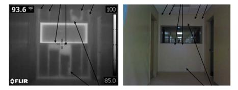
**Fig. H4.5** Loss of thermal barrier continuity through voids at missing insulation and thermal bridging through studs and air leakage under induced pressure differential. Note straight edge and irregular shape anomalies. Source: TMI Air Barrier Testing
