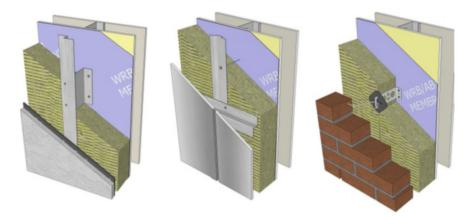
Fig. C.7 Non-proprietary bracket and clip fastening systems – exterior cavity insulation over steelframed structure (EIFS). Alternative installation methods including clip and rail, screw fastened with long screws, and brick ties
