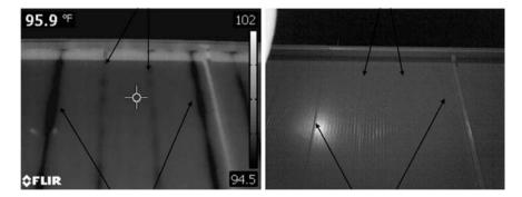
**Fig. H4.2** Loss of thermal barrier continuity due to thermal bridging through metal edges of insulated metal panel joints and air leakage under induced pressure differential through insulated metal panel joints. Note curved/puddle shape anomalies. Source: TMI Air Barrier Testing
