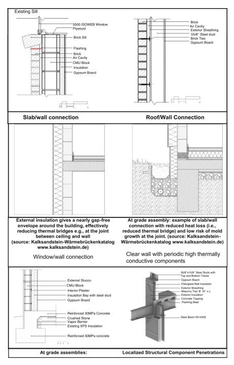
Fig. 8.7 Examples of thermal bridges
