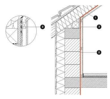
Fig. F.17 Wall/ceiling: (1) air barrier, (2) interior plaster, (3) adhesive, tape, plaster base
