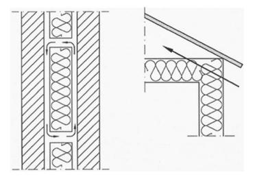
**Fig. 8.4** Convective thermal bridge in a cavity wall where the insulation does not fill the cavity completely and in a wall/roof joint where the wind can blow through part of the insulation. Arrows indicate air flows. (Source: Olsen and Johannesson 1996)
