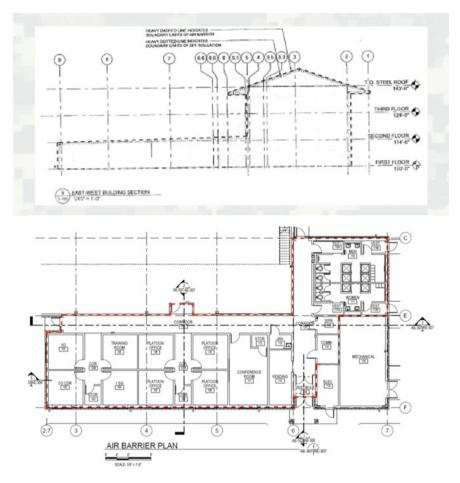
Fig. 9.2 Air barrier boundaries shown on a building section (a) and a plan (b)
