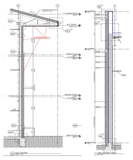
Fig. F.28 Two examples of stud cavity walls showing the air, vapor, and water control layers
