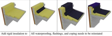
Add rigid insulation to the rear and top of the parapet as well as the cavity if possible
