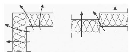
Fig. 8.3 Geometrical thermal bridges. Arrows indicate heat flows. (Source: Olsen and Johannesson 1996)
