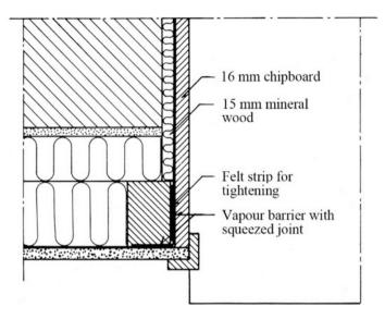
Fig. 6.4 Additional insulation placed behind new opening reveal linings to reduce cold bridges around windows
