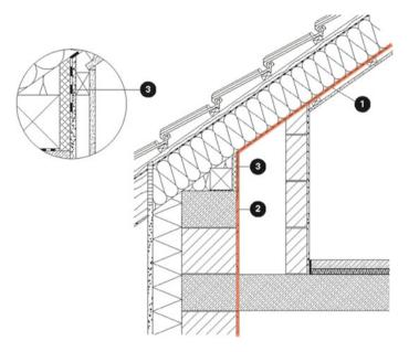
Fig. F.18 Wall/ceiling connection with a jamb: (1) air barrier, (2) interior plaster, (3) adhesive, tape, plaster base
