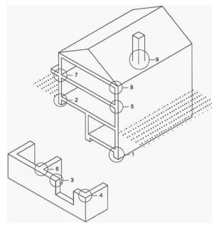
Fig. 8.2 Typical occurrence of thermal bridges in a building. (Source: Olsen and Johannesson 1996)
