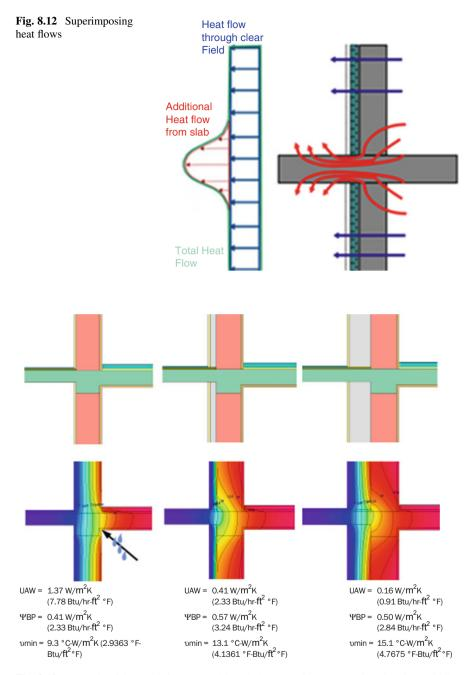
**Fig. 8.13** Example of thermal bridge created by a balcony. Left: prerenovation situation; middle: conventional insulation thickness; right: well-insulated wall with  $\geq 20$  cm of insulation
