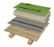
In this option the insulation layer is installed above the rafters, without thermal bridges. The rafters are visible from inside. For static rand optical reasons, it is recommended to have a wooden construction as a first layer. On a first rain protection, the insulation boards have to be fixed by screws in the rafters beyond. Then the substructure and the roof covering follow.
