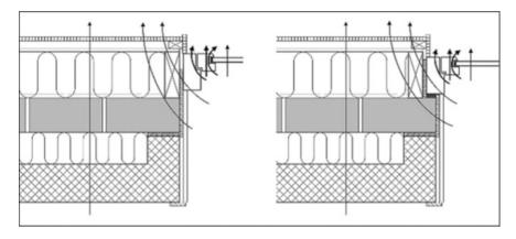
**Fig. 6.8** Example on how a window may be positioned in an externally insulated wall. Cold bridges are reduced by use of a thin insulation layer behind reveal linings and positioning the thermal glazing in plane with the additional insulation. To the right, the window is changed to a slightly larger one allowing more daylight. The arrows in the figure indicate the (reduced) energy loss at cold bridges. (Source: Nørregaard et al. 1984)
