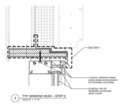
Fig. E.6 Step-by-step illustration of window head installation (Step 2)
