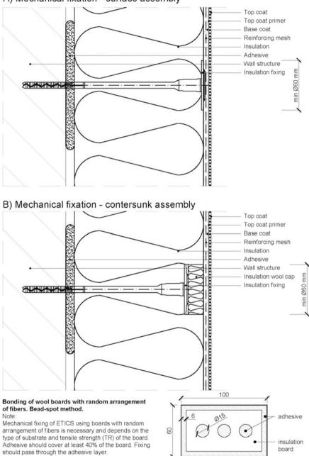
A) Mechanical fixation - surface assembly
