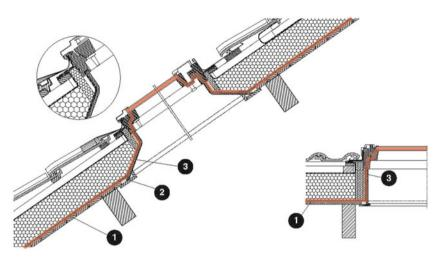
Fig. F.9 Roof with skylights - above rafter: (1) air barrier, (2) tape, corner tape, (4) skirt board
