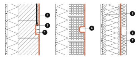
**Fig. F.26** Electrical conduits: (1) electrical installation box, (2) sealing plugs, (3) plaster, (4) airtight electrical installation box, (5) installation housing, (6) air barrier, (7) installation level
