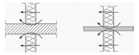
Fig. 8.5 Constructive thermal bridges. Arrows indicate heat flows. (Source: Olsen and Johannesson 1996)
