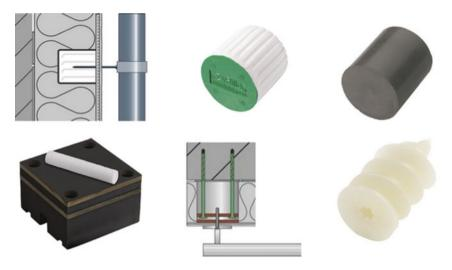
Fig. 8.8 Examples of smaller penetrations: mounting devices to be integrated in insulation layer to give support to railings, shading devices, small roofs, etc., to be mounted outside of insulation layer
