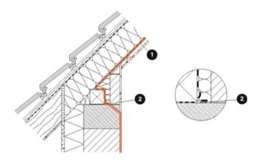
Fig. F.16 Eaves – between-rafter insulation: (1) air barrier, (2) adhesive
