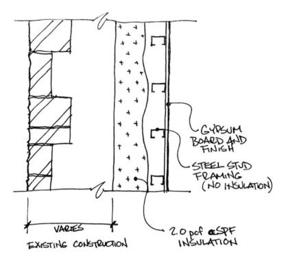
Fig. C.23 Existing masonry with spray foam interior insulation
