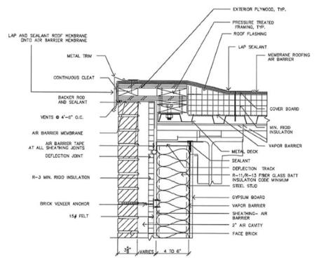
**Fig. F.3** Details of external air barrier for brick veneer wall design, air cavity, R-3 continuous rigid insulation, 15# felt, sheathing air barrier, stud backup, vapor barrier, and gypsum drywall interior finish: (**a**) roof edge; (**b**) parapet; (**c**) floor slab; (**d**) window head; (**e**) window jamb; (**f**) window sill; (**g**) foundation
