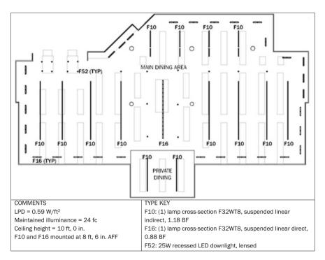
Fig. G.1 Sample schematic lighting layout (not to scale)
