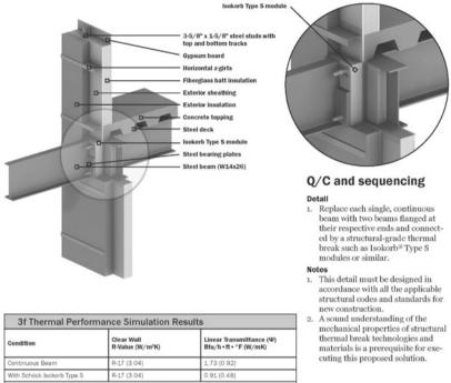
As-built transmittance – Lower tertoff transmittance = Best-case thermal-1.73-0.910 = 0.820 Btu/hft\*F
