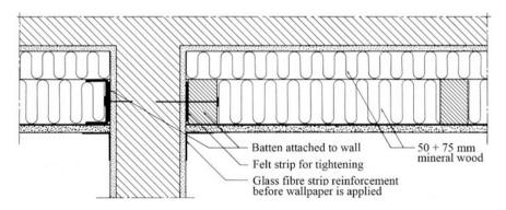
Fig. 6.3 Detail of internally insulated façade around adjoining partition (perpendicular to façade)
