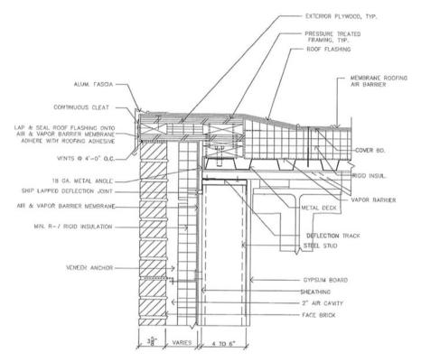
**Fig. F.1** Conceptual details of an external air barrier for building with a brick veneer wall, a pitched shingle roof and a metal roof: brick, 2 in. cavity, continuous insulation, air/vapor barrier, sheathing, a steel stud backup wall, and a gypsum drywall interior finish. (a) Roof edge; (b) parapet; (c) floor slab; (d) penetration; (e) window head; (f) window jamb; (g) window sill; (h) foundation; (i) shingle roof; (j) metal roof
