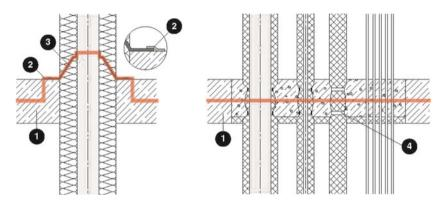
Fig. F.27 Pipe penetration: (1) ceiling, (2) tape, (3) sleeve, molded part, (4) cable tie
