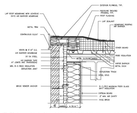
**Fig. F.2** Conceptual details of external air barrier for building brick with veneer wall design, with 2 in. cavity, 1 in. insulating sheathing (air barrier), R-11/R-13 (maximum), unfaced fiberglass batts in stud space and stud backup wall: (a) roof edge; (b) parapet; (c) floor slab; (d) window head; (e) window jamb; (f) window sill; (g) foundation
