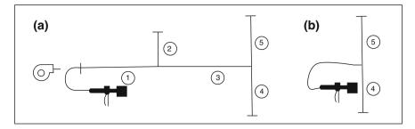
**Fig. 12.9** Ductwork layout and instrumentation, for example: (a) pressurizing entire system; (b) pressurizing sections 4 and 5 combined (note: [.....] denotes a temporary seal of a duct opening)
