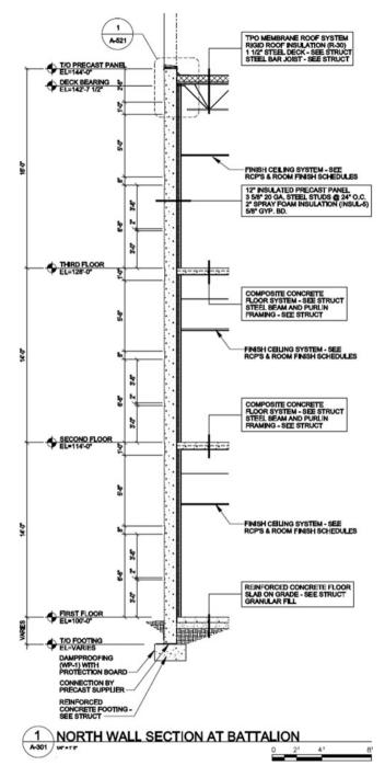
Fig. F.30 First of two sections for a precast concrete wall assembly
