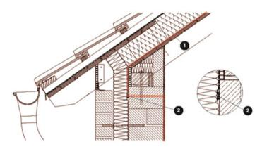
Fig. F.15 Eaves – above rafter insulation, continuous rafters, lined compartments: (1) air barrier, (2) adhesive
