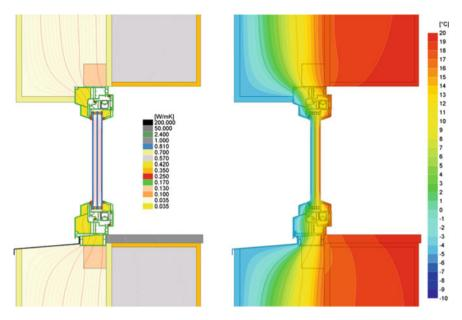
Fig. 6.9 Example of window installation within exterior finish insulation system (EFIS) (reproduced with permission from PHI)
