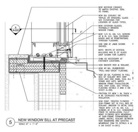
Fig. E.8 Illustration of window sill installation
