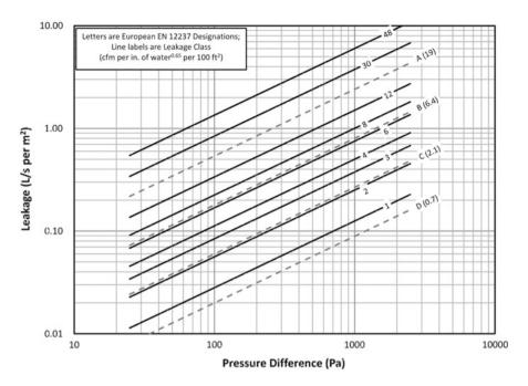
Fig. 12.5 Relationship between European air tightness classes (dashed lines) and ASHRAE leakage classes (solid lines) in SI units
