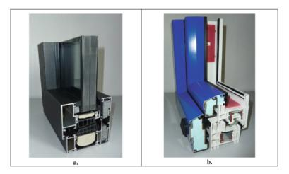
Fig. 7.5 Examples of high performance windows with frames made from different materials: (a) aluminum frame with full thermal separation; (b) plastic PVC frame with additional cladding including insulation layer
