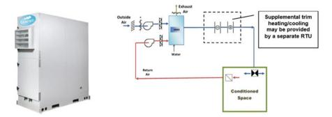
Fig. 12.4 Hybrid DOAS using indirect evaporative cooling and heating with energy recovery ventilation (ERV) (USACE 2016)
