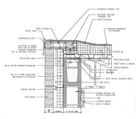
Fig. F.4 Details of external air barrier design of brick veneer wall, cavity, rigid insulation, air and vapor barrier, concrete block backup, gypsum board: (a) roof edge; (b) parapet; (c) floor slab; (d) wall detail; (e) window head; (f) window jamb; (g) window sill; (h) foundation
