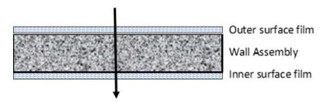
Fig. 6.1 Simplified schematic of heat transfer through wall (roof) assembly
