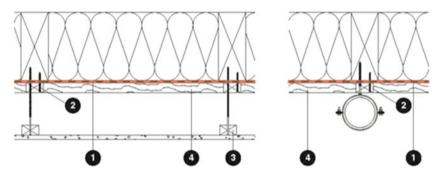
Fig. F.13 Suspension: (1) air barrier, (2) laths, (3) ceiling suspension, (4) loadbearing lath
