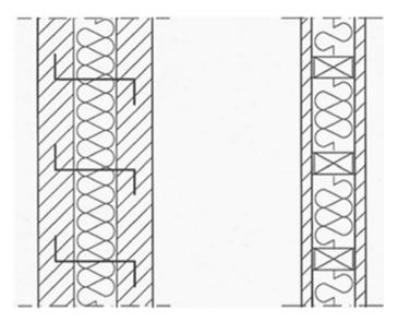
Fig. 8.6 Typical systematic thermal bridges. (Source: Olsen and Johannesson 1996)
