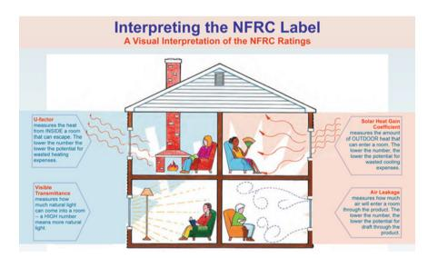
Fig. 7.4 Primary window energy performance elements at work
