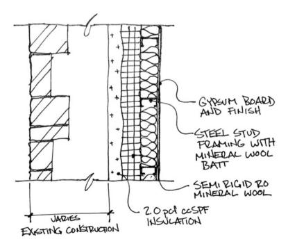
Fig. C.24 Existing masonry with hybrid interior solution (spray foam and mineral wool insulation)
