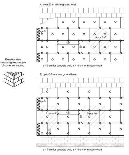
Fig. C.3 Example of mechanical fastening patter for large mineral wool boards
