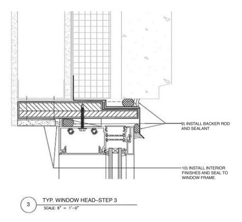
Fig. E.7 Step-by-step illustration of window head installation
