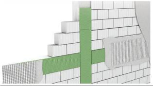
XPS boards reducing thermal bridges by concrete studs and ceilings in monolithic walls
