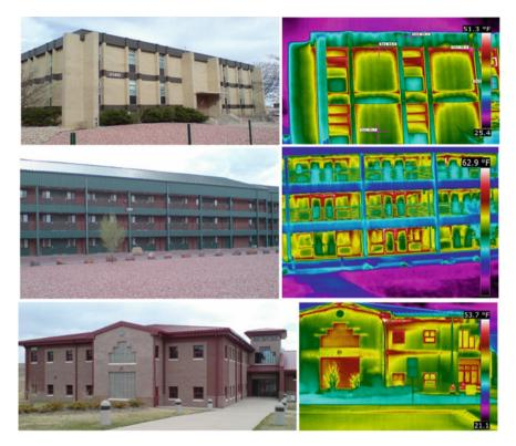
Fig. 8.1 Examples of thermal bridges: parapets, doors, slabs
