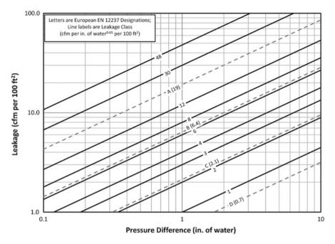
Fig. 12.6 Relationship between ASHRAE leakage classes (solid lines) and European air tightness classes (dashed lines) in IP units
