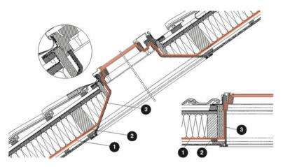
Fig. F.8 Roof with skylights: (1) air barrier, (2) tape, corner tape, (3) skirt board
