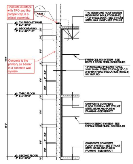
Fig. F.31 Second of two sections for a precast concrete wall assembly
