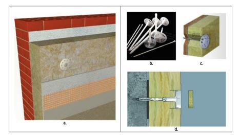
**Fig. C.8** Mechanically attached insulation: (a) mechanically fastened mineral wool board, (b) fasteners, (c) cross-section, (d) recessed mechanical fastener with insulation disc
