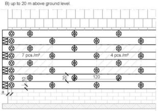
a > 5 cm for concrete wall, a >10 cm for masonry wall
