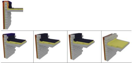
Remove capping, flashings, and roof coverings to expose CMU wall and roof insulation
