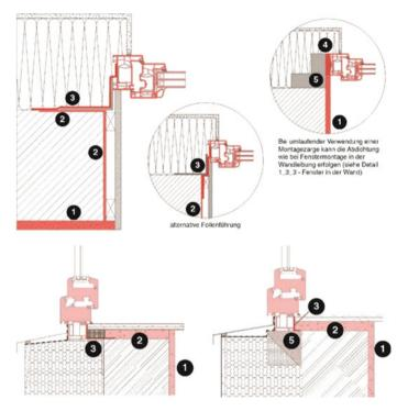
**Fig. F.21** Window installed within the wall: (1) interior plaster; (2) smooth finish (if needed); (3) foil joint seals; (4) deviation from the standard installation, e.g., multifunction adhesive strips; (5) subframe
