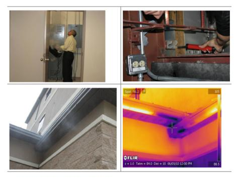
Preparing the building for an airtightness test should follow air barrier test standards (e.g., USACE/ Air Barrier Association of America's airtightness test protocol) while using the smoke tracer; infrared thermography can also be helpful in determining existing leakage problems.
