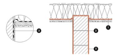
Fig. F.19 Inner wall/roof: (1) air barrier, (2) adhesive or tape (fleece laminated), plaster base, (3) plaster
