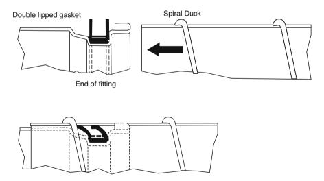
Fig. 12.7 Double-lipped gasket connection of round ducts (unassembled and assembled)
