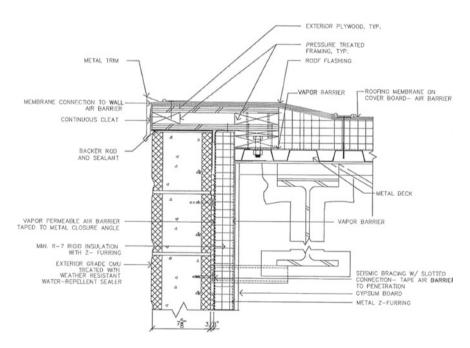
Fig. F.5 Details of external air barrier single wythe concrete block with R-7 interior insulation. Commercial grade spun-bonded polyolefin air barrier, rigid insulation, vapor barrier, interior drywall: (a) roof edge; (b) parapet; (c) floor slab; (d) single wythe CMU; (e) window jamb; (f) window sill; (g) foundation
