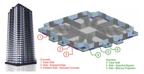
Fig. 8.14 Example of calculation of the overall heat transmission rate of any specific part of the enclosure by summing the heat transmission from each element
