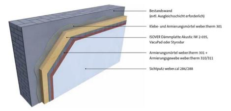
(1) Existing wall; (2) glue and reinforcement mortar; (3) mineral wool insulation board; (4) reinforcement mortar and mesh; (5) final rendering
