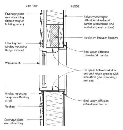
Fig. E.1 Example of window installed as part of drainage wall system. (Illustration taken from *Residential Windows: a Guide to New Technologies and Energy Performance*)
