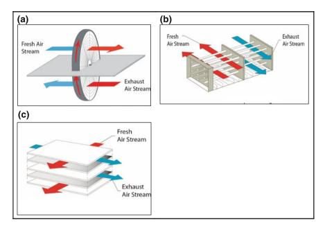
Fig. 12.2 Typical heat recovery components: (a) rotary air-to-air energy exchanger, (b) heat pipe heat exchanger, and (c) fixed plate cross-flow heat exchanger
